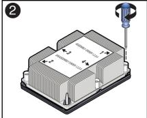
g. Using a 12.0 in-lbs (inch-pounds) torque driver with a Torx T30 bit, tighten the processor-heatsink module to the socket. First, fully tighten captive nuts 1 and 2. Then fully tighten nuts 3 and 4 [2]
