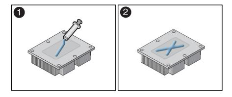
**Note -** Do not distribute the TIM; the pressure of the heatsink will do so for you when you install the heatsink.
