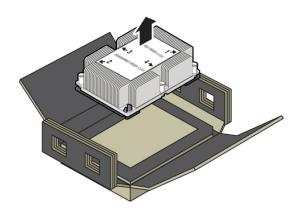
d. Align the processor-heatsink module to the processor socket bolster plate on the motherboard, matching the pin 1 location [1].
