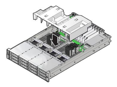
3. Rotate the HBA super capacitor tray down and in to its closed position.
