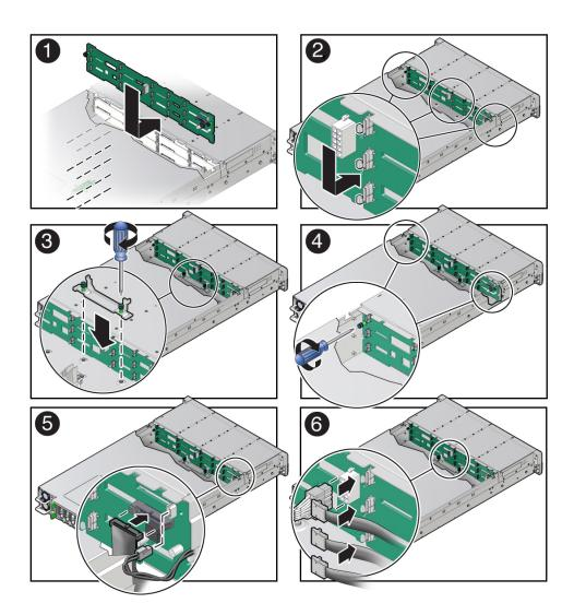
2. Lower the backplane bracket into the server, and using a Torx T25 screwdriver, tighten the spring-mounted screws to secure the bracket to the chassis [3].
