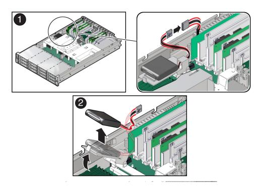
3. Rotate the PCIe card locking mechanism, and lift up on the PCIe HBA card to disengage it from the motherboard connectors [1].
