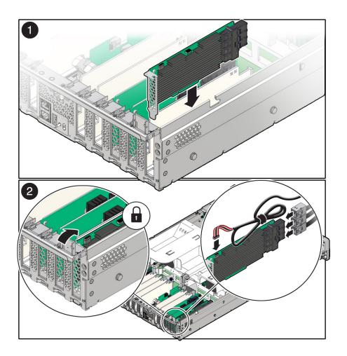
3. Connect the super capacitor cable to the internal HBA card, and reconnect the SAS cables that you unplugged during the removal procedure [2].
