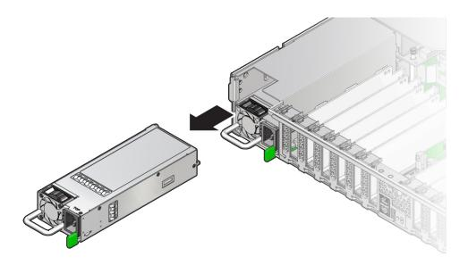
7. Pull the power supply out of the chassis.
