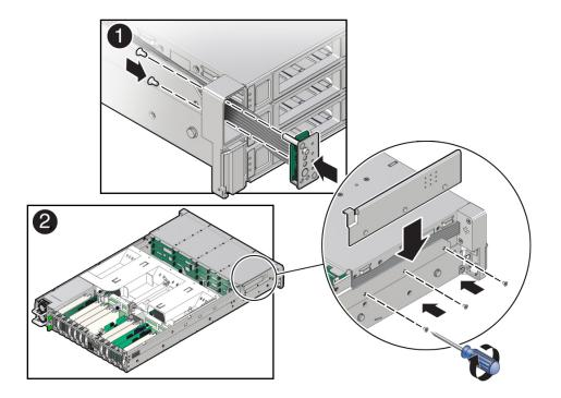
b. Install the LED indicator module cable by carefully pulling the cable through the cable trough along the left side of the chassis.
