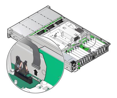
3. Remove the three No. 2 Phillips screws that secure the FIM cable and Temp Sensor Access cover to the chassis [1].
