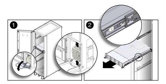
4. While the release latch covers are in the open position, slowly pull the server forward until the slide-rails latch into a locked position [2].
