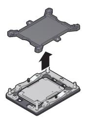
b. Install a processor into the socket from which you removed the processor socket cover.
