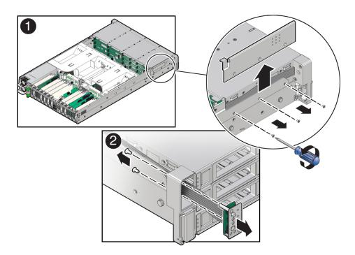
Lift up and remove the FIM cable and Temp Sensor Access cover from the FIM cable and Temp Sensor Access cover slot [1].
