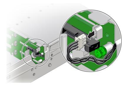
4. Remove the three No. 2 Phillips screws that secure the FIM cable and Temp Sensor Access cover to the chassis [1].
