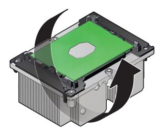
b. While holding down the processor-heatsink modules by the edges, insert a flat blade screwdriver into the TIM breaker slot.
