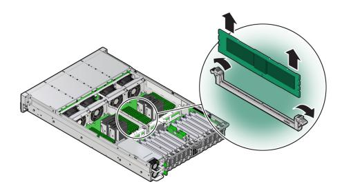
4. Replace each faulty DIMM with another DIMM of the same size and type.
