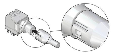
ii. Push the light pipe onto the housing until the clips latch in the holes.
