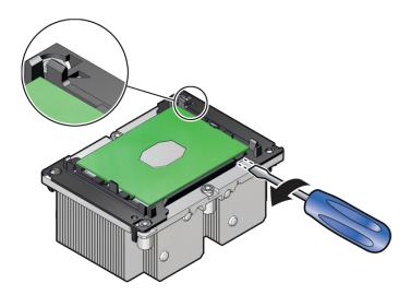
c. Use a rocking motion to gently pry the corner of the processor carrier away from the heatsink.
