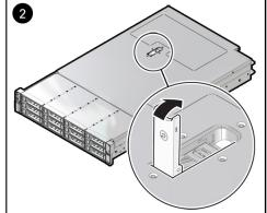
4. Use a Torx T15 screwdriver to turn the release button latch counter-clockwise to the locked position.
