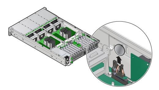
3. Lift the battery up and out of its retainer.
