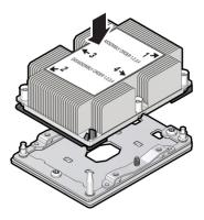
f. Ensure that the processor-heatsink module lies evenly on the bolster plate and that the captive screws align with the threaded socket posts [1].
