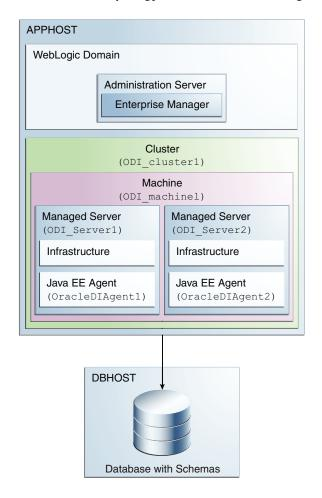
Figure 1-2 Standard Installation Topology for an ODI Java EE Agent
