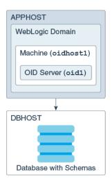
Figure 1-2 Standard Topology for Oracle Internet Directory Collocated Installation
