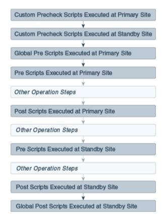
Figure 2-5 Execution Sequence of Scripts for Failover Operation
