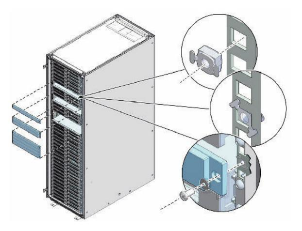
Figure 7-4 Removing the Filler Panels
