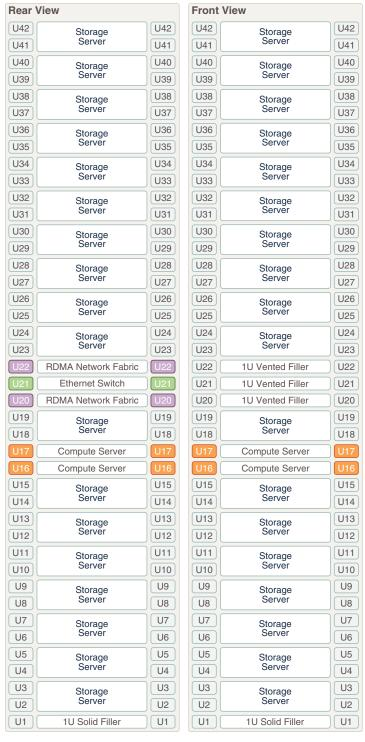
Figure 19-2 shows the front and rear views of a Recovery Appliance RA21 and X8M minimum configuration.
