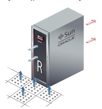
Figure 2-7 Typical Data Center Configuration for Perforated Floor Tiles
