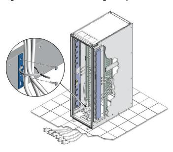
Figure 6-8 Power Cord Routing Example
