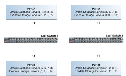
Figure 25-2 Connections Between Database Servers and Storage Servers and Leaf Switches
