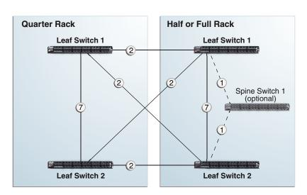
Figure 25-6 Leaf and Spine Switch Connections Between a Quarter Rack and a Half or Full Rack
