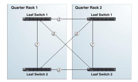
Figure 25-5 Leaf Switch Connections Between 2 Quarter Racks
