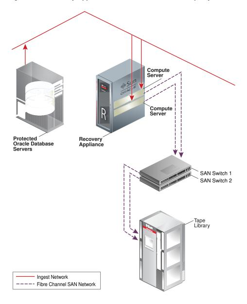
Figure 3-7 Recovery Appliance Connection to an Oracle Tape System
