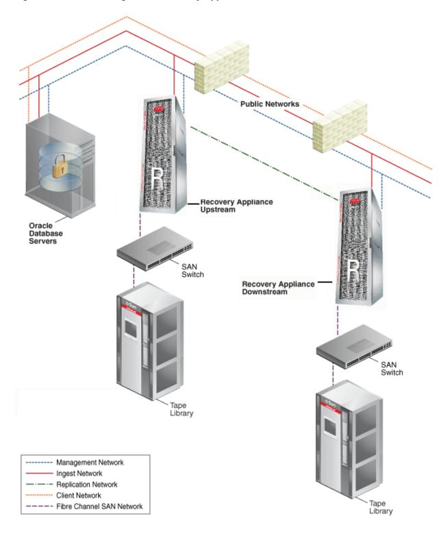
Figure 3-5 Network Diagram for Recovery Appliance
