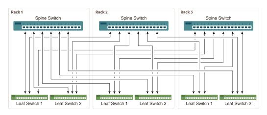
Figure 24-1 Connections Between Spine Switches and Leaf Switches for up to 8 Racks
