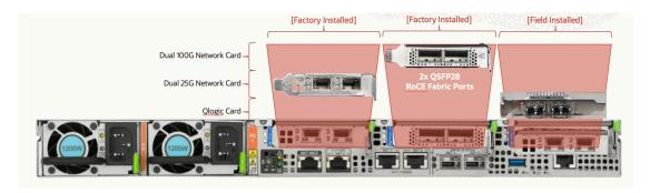
Maximum of two 25G ports for ingest and two 25G ports for replication, per compute server
