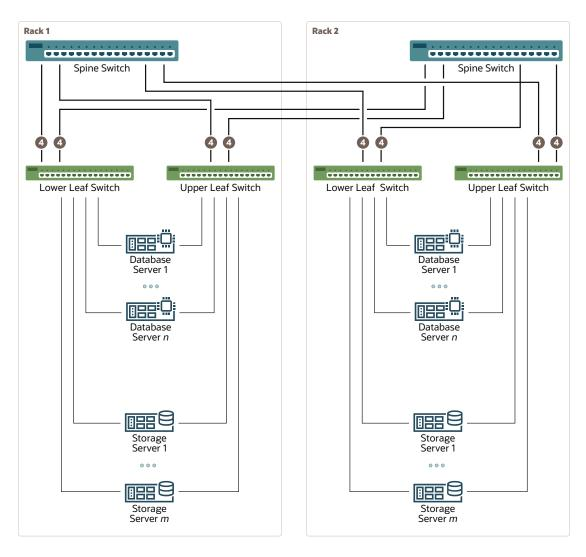
As shown in the preceding graphic, each leaf switch in rack 1 has the following connections:
