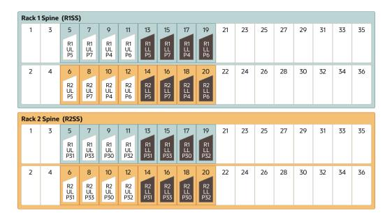
The following table describes the cable connections for the first spine switch (R1 SS) when cabling two racks together:
