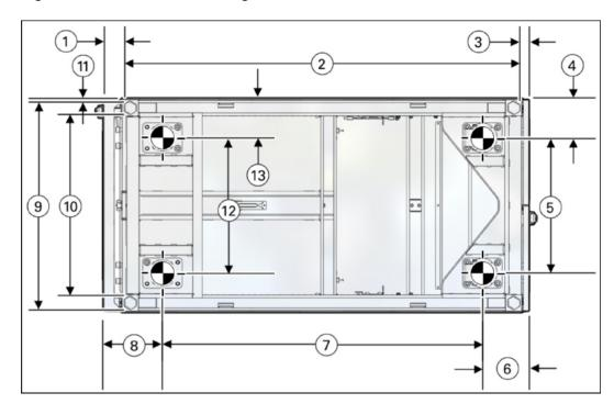
Figure 6-5 Location of Leveling Feet on ZDLRA Rack X7 or later
