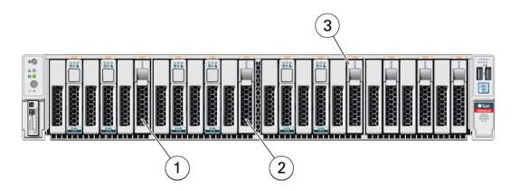
If you have the default configuration of NVMe drives (seen as  $pd_00$ ,  $pd_01$ ,  $pd_03$ ,  $pd_04$ ,  $pd_06$  and  $pd_07$  from the host), you can expand storage by adding three (3) NVMe drives.
