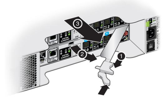
For the DE2-24C or DE2-24P, using your thumb and forefinger, squeeze the release button [1] toward the locking lever hole to release the lever [2]. Grasp the lever and remove the I/O module from the chassis.
