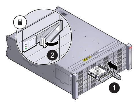
d. Repeat steps a through c until all of the empty drive slots in the storage shelf are filled with the new drives
