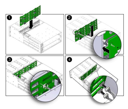
c. Position the disk midplane module against the disk drive cage, tilting the top slightly forward so that it fits over the top-most standoff on the left side and then position board so that it fits over the remaining 12 standoffs, then push downward on the board to engage the standoffs [2] as shown in the previous figure.
