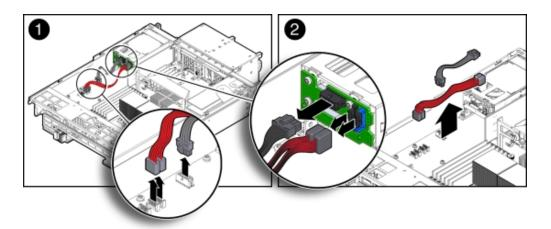
b. Disconnect the power cable and HDD cables from the boot disk backplane [2] as shown in the previous figure.
