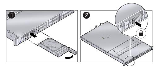
Power on and remount the replacement drive. Type the following command from the host:
