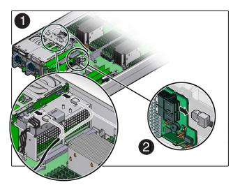
Install the replacement SAS cable to the rear disk drive backplane [1] and the SAS card [2] as shown in the following figure.
