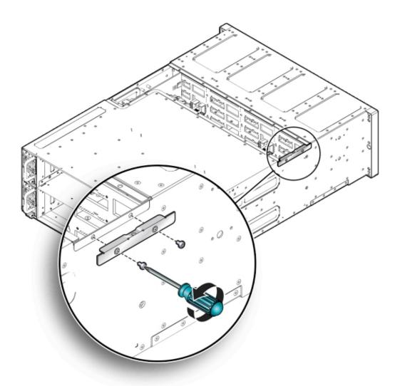
6. Remove the power distribution board.
