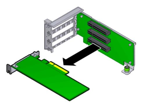
b. Place the PCIe card on an antistatic mat.
