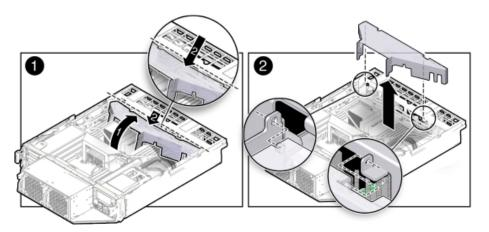
b. Grasp the left end of the plastic air duct with your left hand to hold it at a 45 degree angle, and with your right hand press gently down on the middle of the air duct until it bends enough to disengage its hinges from their sockets and allow removal of the air duct [2] as shown in the previous figure.
