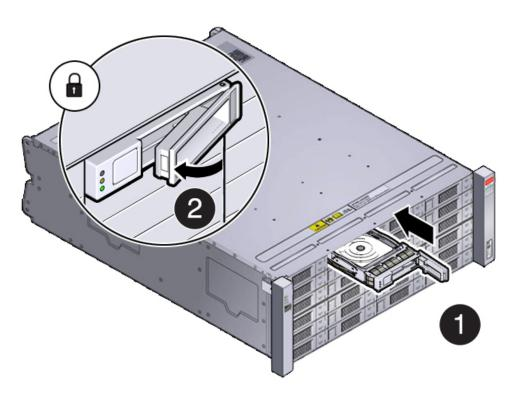
• For the DE2-24P, open the drive lever on the replacement drive. Slide the drive into the drive slot until it engages with the backplane connector and then close the lever to fully seat the drive and lock it into place as shown in the following figure.
