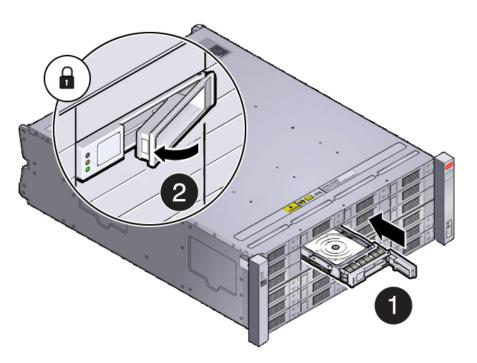
**d.** Repeat steps a through c until all of the new drives are installed in the storage shelf.
