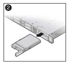
4. Align the replacement drive with the drive slot.
