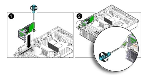
**d.** Tighten the three green captive Phillips screws that secure the PCle riser to the chassis [2] as shown in the previous figure.
