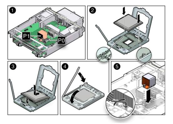
b. Carefully lower the end of the CPU with the alignment tabs into the socket, support the raised end of the CPU with the index finger on your other hand, and lower the CPU into the socket [3] as shown in the previous figure.
