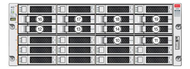
• If your system is running **Oracle Database Appliance software release 18.7, 18.8, 19.6 or later version**, 7.68 TB SAS SSDs can be used for storage expansion (1.6 TB SSDs are no longer available). However, this means that you must also replace any existing 1.6 TB SSDs with 7.68 TB SSDs, perform clean-up, redeploy the appliance software, and restore the database from a backup. You cannot have both types of drives in the storage shelf.
