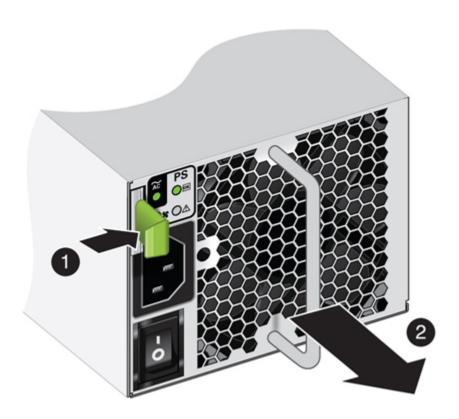
• For the DE2-24C or DE2-24P, push the ejector release button [1], grasp the power supply ejector handle and rotate it to the open position [2] as shown in the following figure. Slide the power supply out of the chassis.
