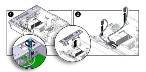
**b.** Disconnect the two secondary HBA PCIe card cables and remove the cables [2] as shown in the previous figure.
