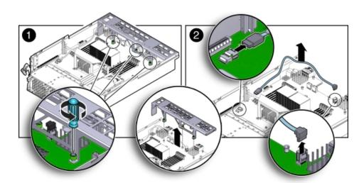
**b.** Disconnect both cable connectors from the motherboard and remove the cable [2] as shown in the previous figure.
