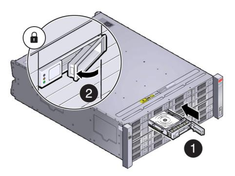
d. Repeat steps a through c until all of the new drives are installed in the storage shelf.
