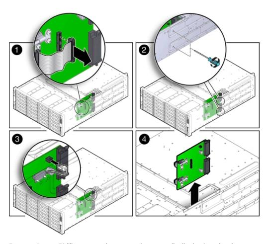
**b.** Remove the two Phillips screws that secure the power distribution board to the chassis [2] as shown in the previous figure.
