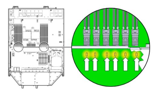
If the DIMM fault LED is off, the DIMM is operating properly.
