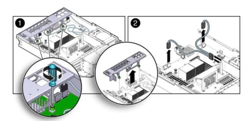
**b.** Disconnect the two cables from the primary HBA PCIe card and remove the cables [2] as shown in the previous figure.
