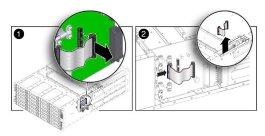
**4.** Disconnect the HDD ribbon cable connector located on the disk midplane module [2] as shown in the previous figure.
