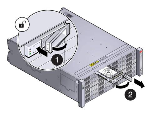
• For the DE2-24P, slide the release latch as indicated by the debossed arrow to release the drive lever and then, rotate the lever open and, grasping the drive body, slide the drive out of the storage shelf as shown in the following figure.
