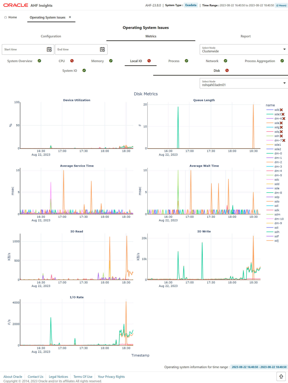
Figure 5-13 Operating System Issues - Metrics - Disk Anomalies
