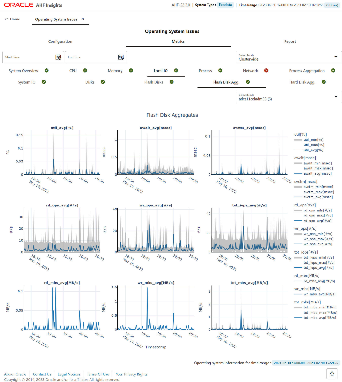
Figure 5-16 Operating System Issues - Metrics - Local I/O - Flash Disk Aggregation
