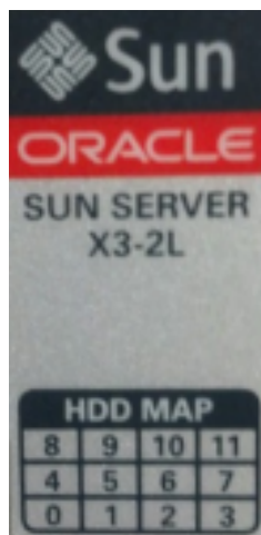
Figure 10-1 Disk Layout in Exadata Storage Server X3-2 Servers
