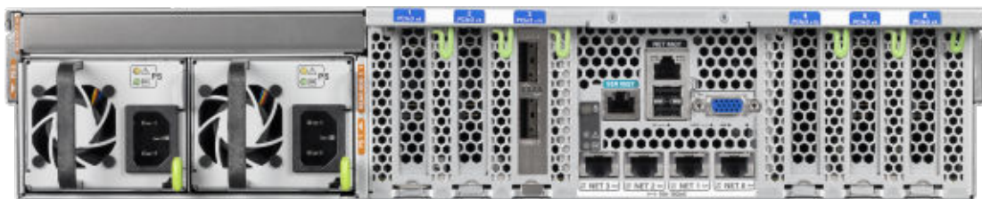
Figure 3-28 Rear View of Extreme Flash Exadata Storage Server X5-2 Servers
