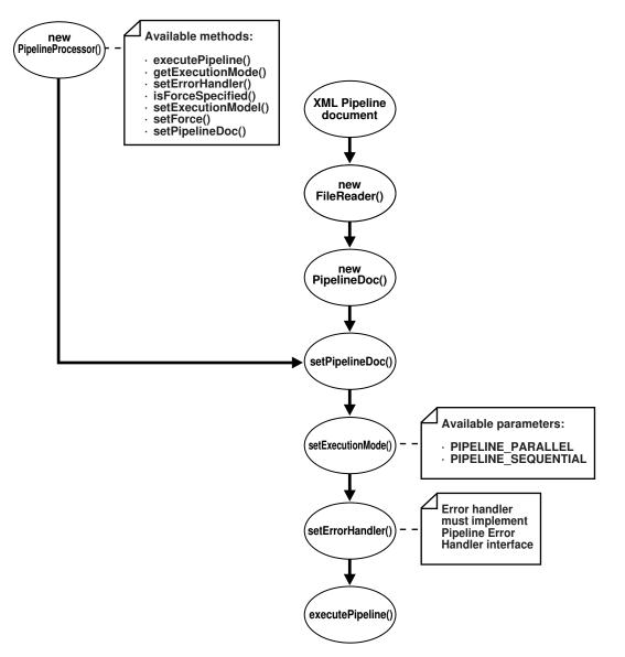
Figure 19-2 Using the Pipeline Processor for Java
