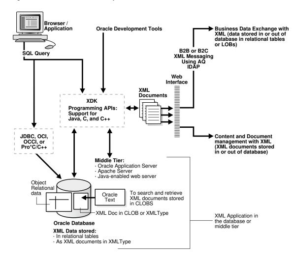
Figure 1-10 Oracle XML Developer's Kit Tools and Frameworks
