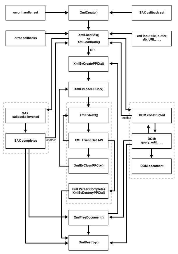
Figure 5-1 XML Parser for C Calling Sequence
