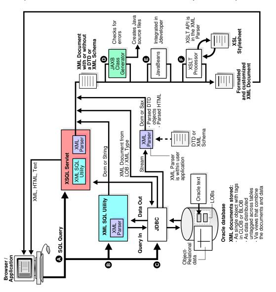
Figure 1-7 Sample XML Processor Built with Java Oracle XML Developer's Kit Components
