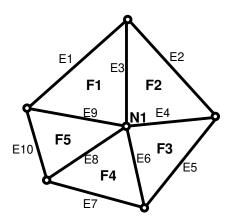
Figure 2-6 shows two cases of the original topology after node N1 is moved. In one case, no reshaping occurs; that is, all edges affected by the movement are specified as straight lines. In the other case, reshaping occurs; that is, one or more affected edges are specified as line segments with multiple vertices.
