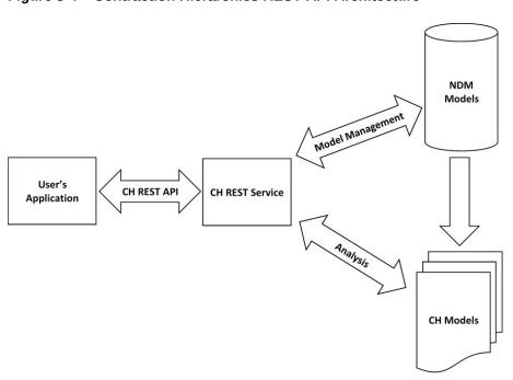
Figure 5-4 Contraction Hierarchies REST API Architecture
