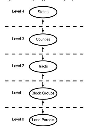
Figure 1-4 Topology Geometry Layer Hierarchy
