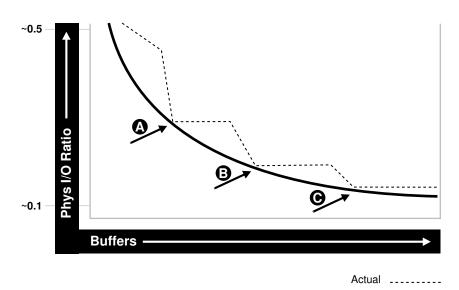
Figure 13-1 Physical I/O Ratio and Buffer Cache Size
