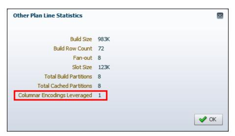
Because Columnar Encodings Leveraged is a positive value and Columnar Encodings Observed is not present, the join group was leveraged.
