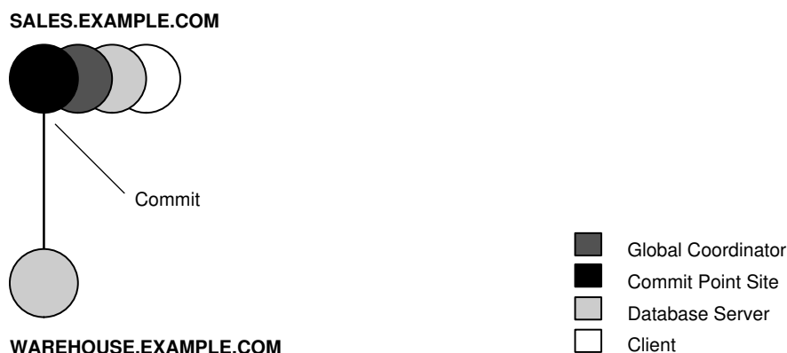
Figure 34-8 Determining the Commit Point Site
