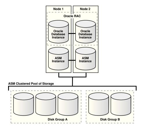
Figure 1-3 Oracle Instances and Oracle ASM Storage
