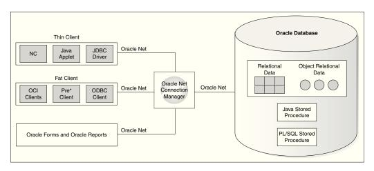
Figure 1-5 Two-Tier Client/Server Configuration
