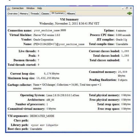
Figure 2-14 The VM Tab of the JConsole Interface
