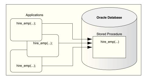
Figure 6-1 Calling a Stored Procedure
