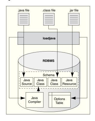
Figure 2-2 Loading Java into Oracle Database
