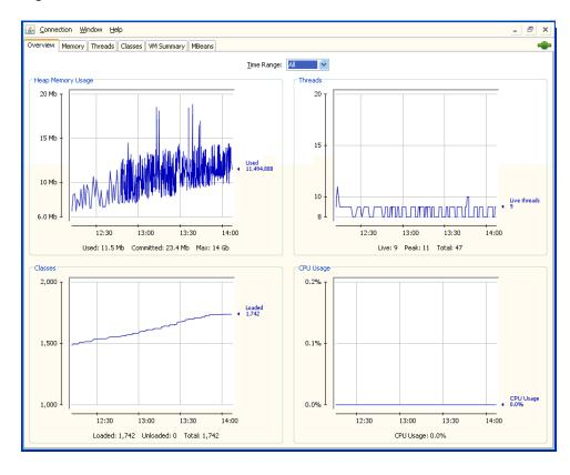
Figure 2-6 The Overview Tab of the JConsole Interface
