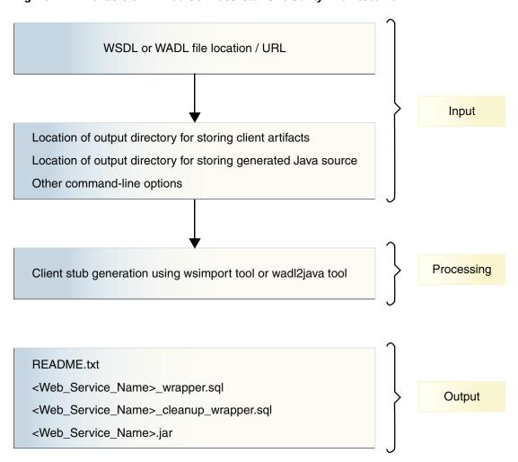
Figure 14-1 Oracle JVM Web Services Call-Out Utility Architecture
