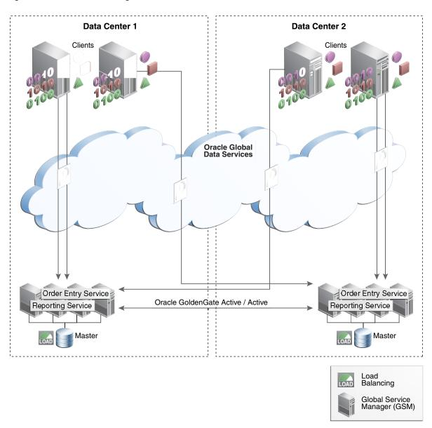
Figure 1-7 Load Balancing in Oracle GoldenGate Multi-Master
