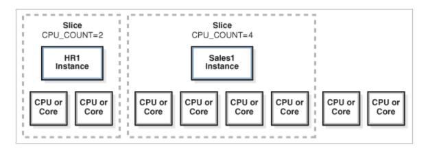
When you implement instance caging, Oracle Database QoS Management can provide recommendations to reallocate CPU resources from one slice to another slice within the same server pool. If you choose to implement the recommendation to modify the instance caging settings, then Oracle Database QoS Management modifies the CPU\_COUNT parameter uniformly for all the database instances running on servers in the server pool.
