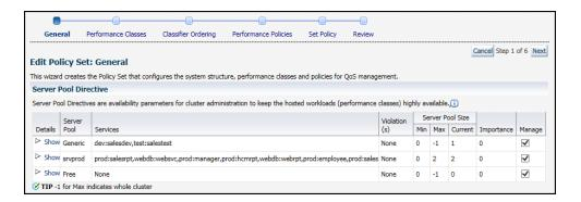
This page lets you specify which server pools are managed by Oracle Database QoS Management. If the Manage box for a server pool is unchecked, then none of the servers, databases or workloads that use that server pool are displayed or managed by Oracle Database QoS Management. The Details column displays any configuration violation details and the corrective action to take to enable the server pool to be managed.
