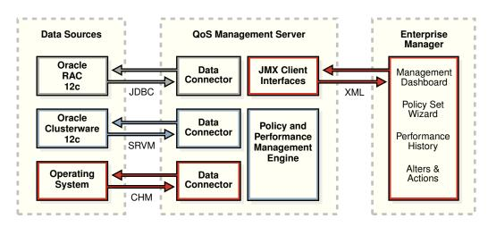
Figure 1-6 Diagram of Oracle Database QoS Management Server Architecture
