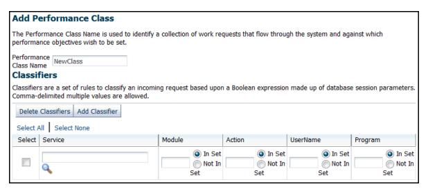
4. In the Classifiers section, enter information to define a rule for classifying work requests. First select a database service, then specify matching values (In Set) for the module, action, UserName, or program name that is associated with the work request using the specified database service. You can also specify exclusion values (Not In Set) for these attributes.
