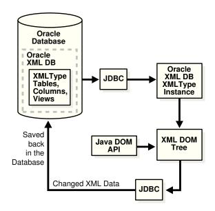
Figure 13-1 Using the Java DOM API for XMLType
