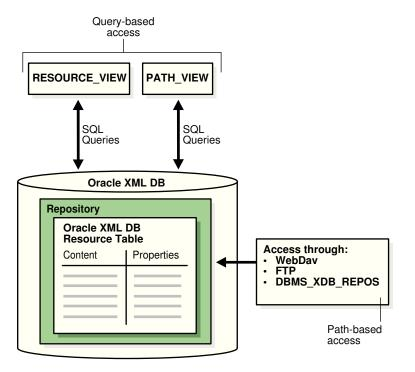
Figure 24-1 Accessing Repository Resources Using RESOURCE\_VIEW and PATH VIEW
