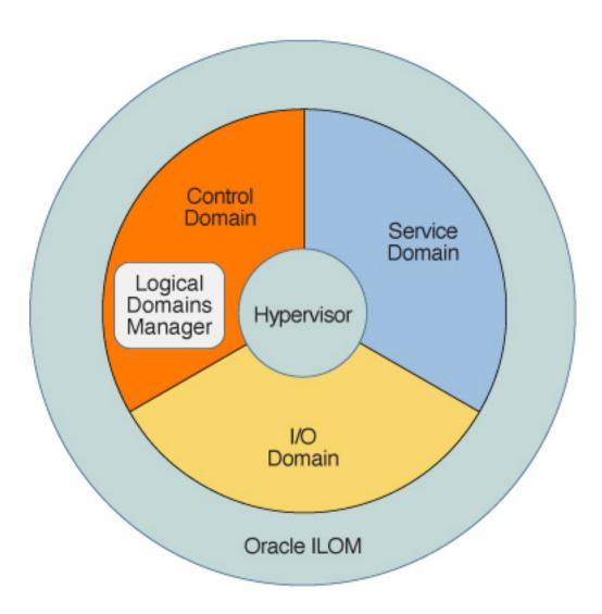
**FIGURE 3** Components of the Execution Environment
