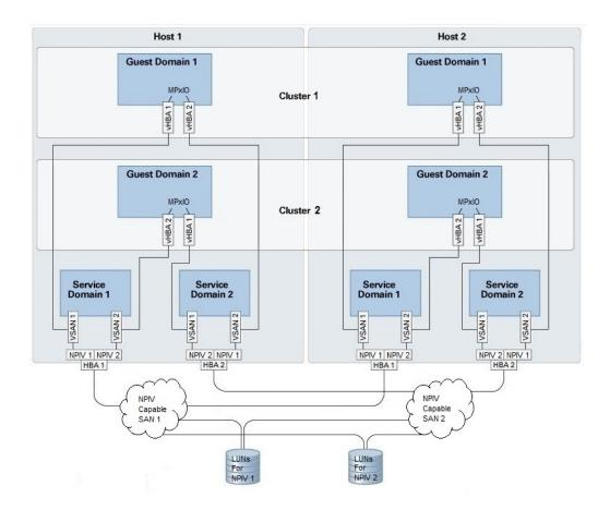
**Note** - Besides cluster nodes with virtual devices for I/O from service domains, a topology where cluster nodes are I/O domains with SR-IOV devices is also supported, including with redundant root domains supplying redundant virtual functions to the I/O domain. For additional information see "SPARC: Guidelines for Oracle VM Server for SPARC Logical Domains as Cluster Nodes" in *Installing and Configuring an Oracle Solaris Cluster 4.4 Environment*.
