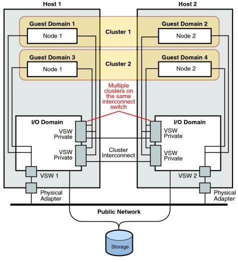
FIGURE 10 SPARC: Clusters Span Two Different Hosts
