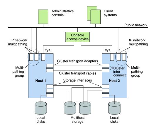
FIGURE 1 Oracle Solaris Cluster Hardware Components
