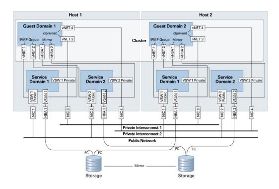
Only one guest domain cluster can be supported per one VSAN/vHBA combination. To add additional guest domain clusters, more VSANs/vHBAs can be created by using different HBA ports. In this configuration, the number of vHBAs on any one VSAN should be only one as there is no access control per vHBA.
