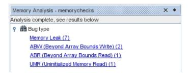
8. When you click on an error type, the errors of that type are displayed in the Memory Analysis Tool window.
