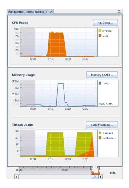
Notice that in the CPU Usage and Memory Usage indicators for the same time period has the single thread performing some activity that uses CPU time and memory. This
