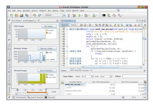
You can also filter for data that meet a certain metric. Right-click on the CPU Time (Exclusive) metrics for work\_run\_usrcpu(). In our example, right-click the 43.07 in the CPU Time Per Function window. Select Show only where > CPU Time (Exclusive) == 43.07. All the rows are filtered away, and only the row whose exclusive CPU time is equal to 43.07 is displayed.
