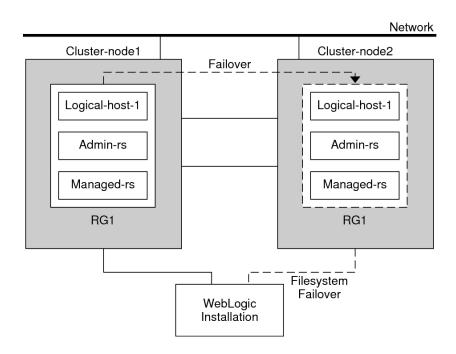
FIGURE 2 HA for WebLogic Server File System Failover Configuration
