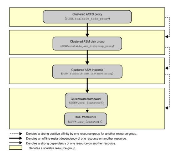
FIGURE 2 Configuration of Oracle ACFS in the Global Zone With Hardware RAID
