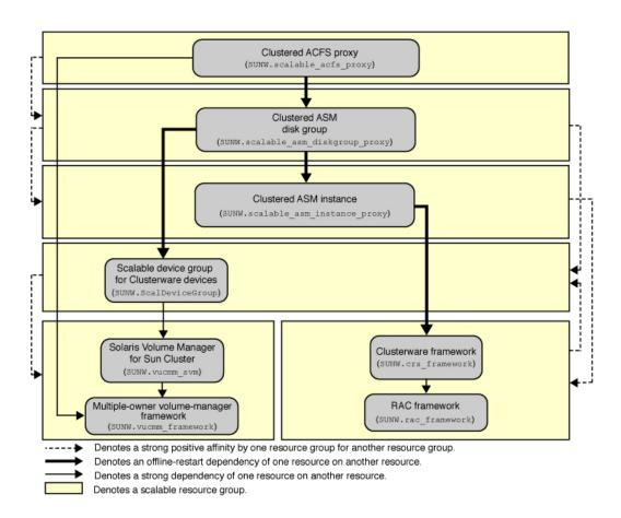
FIGURE 1 Configuration of Oracle ACFS in the Global Zone With Solaris Volume Manager
