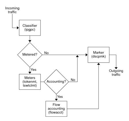
FIGURE 1 Traffic Flow Through the IPQoS Implementation of the Diffserv Model
