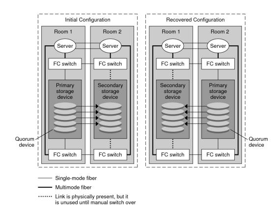
**FIGURE 4-1** Two-Room Configuration With Storage-Based Data Replication
