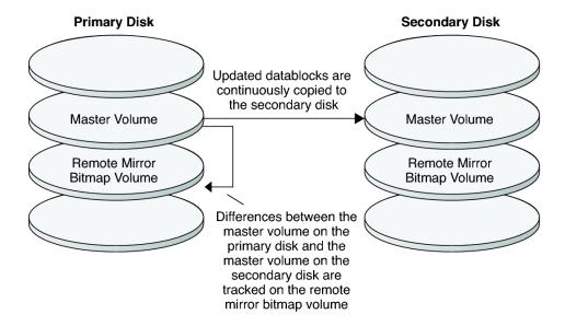
Remote mirror replication can be performed synchronously in real time, or asynchronously. Each volume set in each cluster can be configured individually, for synchronous replication or asynchronous replication.
