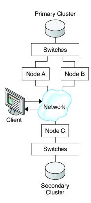
Table A-2 summarizes the hardware and software that the example configuration requires. The Oracle Solaris OS, Oracle Solaris Cluster software, and volume manager software must be installed on the cluster nodes *before* Sun StorageTek Availability Suite software and software updates are installed.
