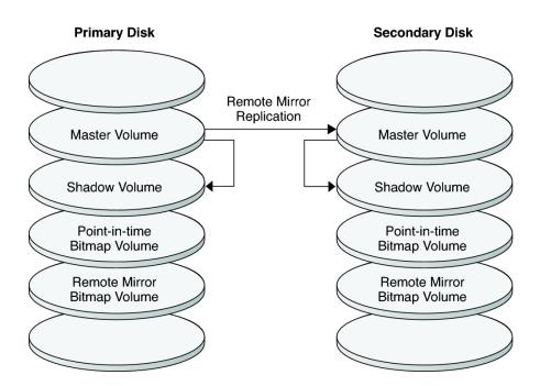
**FIGURE A-3** Replication in the Example Configuration
