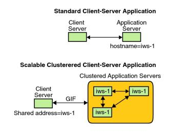
FIGURE 3-5 Fixed Host Name Compared to Shared Address
