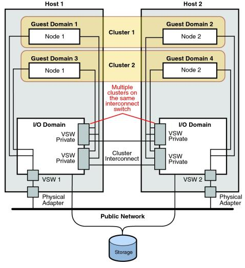
FIGURE 2-10 SPARC: Clusters Span Two Different Hosts
