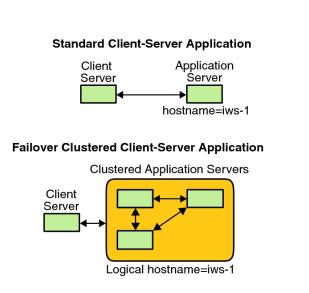
FIGURE 3-4 Fixed Host Name Compared to Logical Host Name
