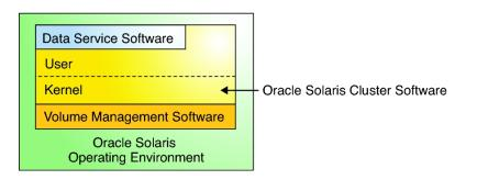
FIGURE 2-2 High-Level Relationship of Oracle Solaris Cluster Components
